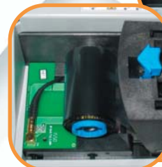
Integrated antenna board fitted inside a Javelin J330i or J430i printer (prior to refitting protective cover)
