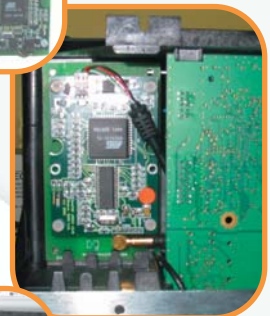
Integrated antenna board fitted inside a Javelin J330i or J430i printer (prior to refitting protective cover)
